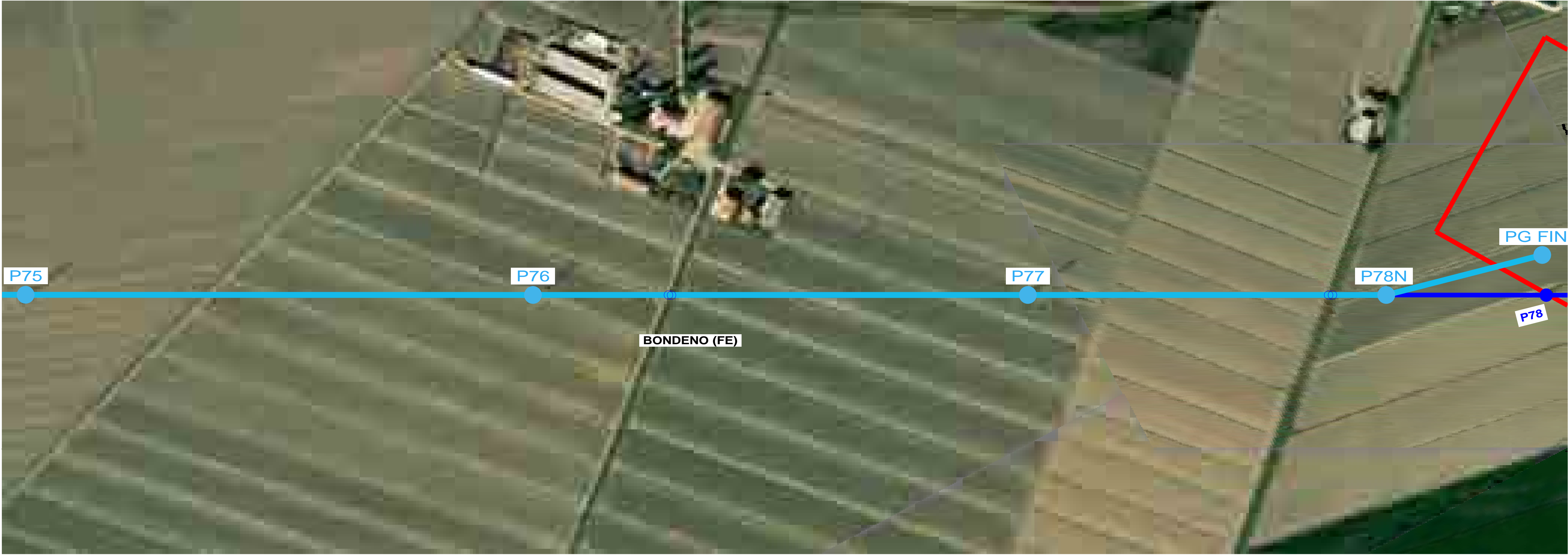
P74 - PG FIN, OPGW 11.5, Displayed MPB Load 2355 (m), Tension as % of Ultimate 13 (%UL) P74 - PG FIN, ACSR 22.8 mm , 3 phases, Displayed MF75 Load 1389 (m), Tension as % of Ultimate 18 (%UL)
