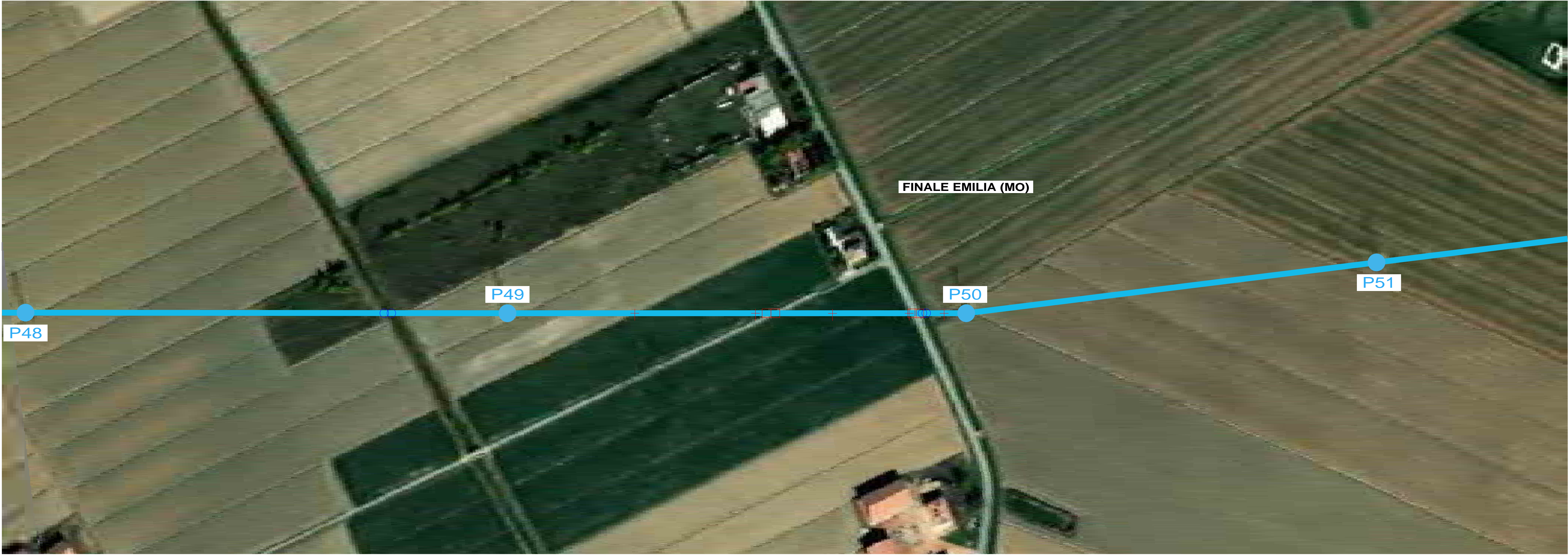
P45 - P74, OPGW 11.5, Displayed MPB Load 2349 (m), Tension as % of Ultimate 13 (%UL) P45 - P74, ACSR 22.8 mm , 3 phases, Displayed MF75 Load 1405 (m), Tension as % of Ultimate 18 (%UL)
